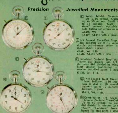
D Sports Model: Measurement divisions are 1/10 second. Outer dial registers up to 30 seconds. Small hand counts up to 15 minutes. 'Start', 'Stop', 'Continue' controls workable from crown. Side button for return to zero. 1 jewel.
