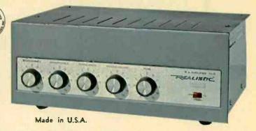
tow Impedance mike — 0.3 mvs;  $600\Omega$  balanced line — 0.1 V. Galn: mike, 123 db; Phono/radio, 83 db. Hum & Noise: 75 db @ rated output, Impedance: mike hi-Imp., 0.5 meg; phono/radio, 1 meg. Speaker Outputs: 4, 16 $\Omega$ ; 25V line, 70V line. Booster/ Tape Recorder: 1 V, low imp. Power: 115 W @ 117 VAC 60 cy. Tubes: 5, 1 rectifier.
